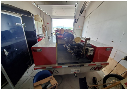
Figure 29: Equipment bays and pump. Vehicle should be assessed to ensure loaded weight is within gross vehicle weight restrictions.
